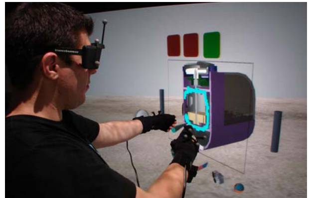
Figure 2. Bimanual asymmetric sketching drawing function in VR prototyping, Benne et al. 2012
